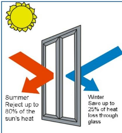
As the sun shines on a building, solar heat gain increases dramatically. The sunny side of a building becomes unbearably hot causing vast temperature imbalances. Air conditioning units must work so much harder to control this rise in temperature with subsequent increase in costs and carbon emissions.
